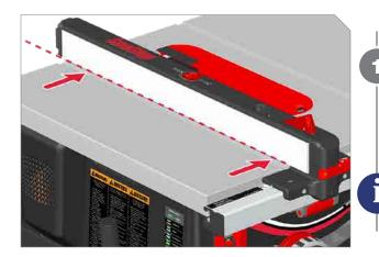
Unlock fence and position with one side flush with a miter gauge slot. Lock fence. Check that face of fence is flush with miter slot edge along whole length. If there is misalignment, continue to next step.
