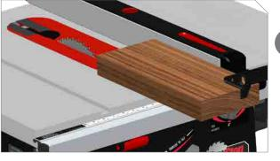
Remove the blade guard and install the riving knife (see page 33). If the non-through cut is a rip cut use the fence.
