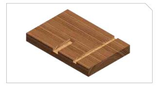
Dado cuts are used to create a slot or trench in the surface of the workpiece. A Dado is cut perpendicular to the grain of the workpiece.
