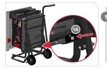
To open mobile cart, grasp both handles and raise cart and saw to upright position. Press lock release lever with right foot (1A) and pull handles toward you.
