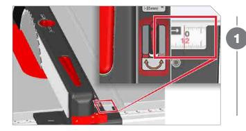
Raise blade fully. Make sure the table is fully retracted. Move fence so its left side rests against right side of blade. If indicator lens reads 0" (0 mm) on ruler, no adjustment is needed. If indicator does not read 0" (0 mm) proceed to next step.
