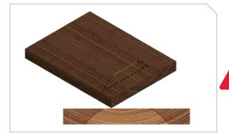
A plunge cut is used to create a slot or opening somewhere other than the edge of the workpiece.
