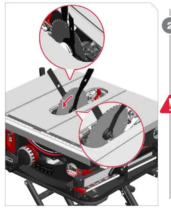
Loosen blade nut with wrenches. Remove nut and washer, change blade, and then reinstall washer and nut. Tighten nut with wrenchesdo not over-tighten. Make sure direction of blade rotation matches direction of teeth, as indicated by red arrow. Reinstall table insert and riving knife/blade guard.
