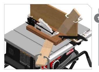
When using a push stick to feed the workpiece, you can use featherboards to maintain the position of the workpiece relative to the fence and table.
