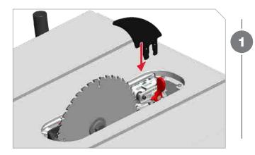
A primary reason to use the riving knife is for non-through cuts where the blade guard and splitter cannot be used.
