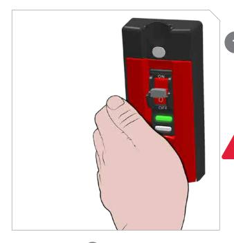
Push paddle in to stop blade. Green status light flashes fast while blade spins down. Saw exits Bypass Mode automatically after blade stops. After all cuts are completed, switch power off.
