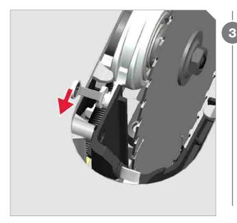
Loosen arbor nut and slide blade over slightly.
