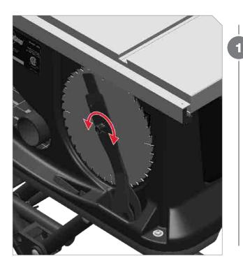
Switch power off and unplug power cord. Remove table insert and riving knife/blade guard. Release wrenches by turning knob 1/2 turn.
