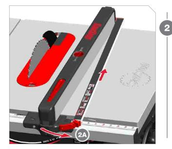
Store low fence on right side of rip fence. Low fence can be used on either side of rip fence. To use low fence on left side of rip fence, pull lever forward (2A) and slide low fence slightly back to unhook rear.
