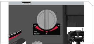
Adjust tilt angle in fractional degree increments by rotating tilt adjustment knob.
