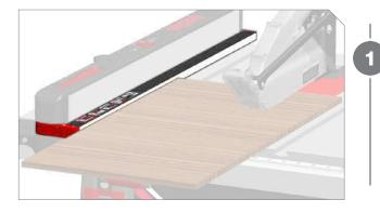
The fence is equipped with a low fence. Use the low fence when cutting thin material or narrow strips of material.
