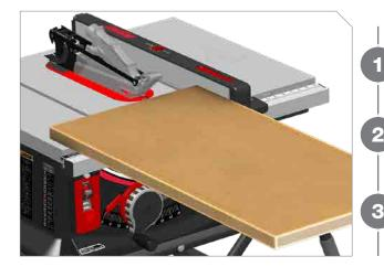
Tilt blade to desired bevel angle and adjust blade elevation to about 1/8" to 1/4" (3 to 6 mm) higher than workpiece.
