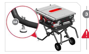
Make sure cart does not wobble. If needed, loosen wing nuts and adjust leveling feet, then re-tighten wing nuts (3A).
