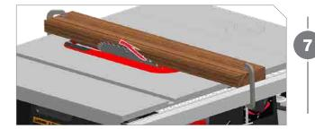
Start motor and slowly raise blade to highest elevation. This will widen slot for beveled cuts up to 45 degrees.
