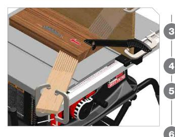
Turn on motor. Slowly raise blade to desired height (partially into or all the way through workpiece).
