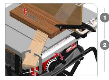
Fully lower the blade. Position the fence at the desired cut width and lock in place. Position the workpiece flat on the table and flush against the fence.
