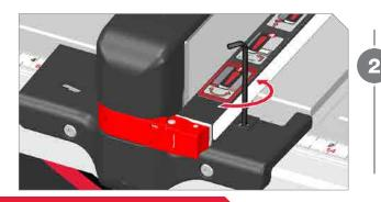
Use a 3 mm hex key wrench to loosen bolt next to indicator lens.
